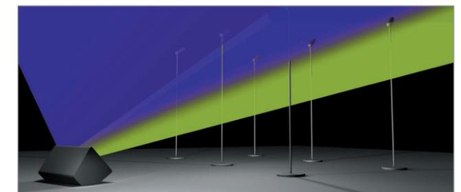
In stage monitor mode, a PS R2 Series loudspeaker yields 100° horizontal coverage at 30° above the centre line, narrowing to 50° horizontal coverage at 25° below the centre line for use when the performers are further away.
