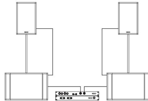
2 x PS15-R2 + 2 x LS18 powered by 2 x DTDAMP4x0.7 (Bridged) + DTD-T-U
