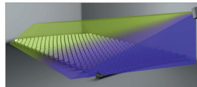
In conventional Front Of House configuration, a PS R2 Series loudspeaker yields 50° horizontal coverage at 25° above the centre line. Rotating the horn expands this to 100° at 50° below the centre line, such that coverage narrows.
